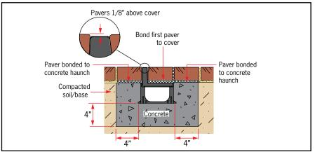
For driveway applications, trench drain **MUST** be surrounded by 4" of concrete.
