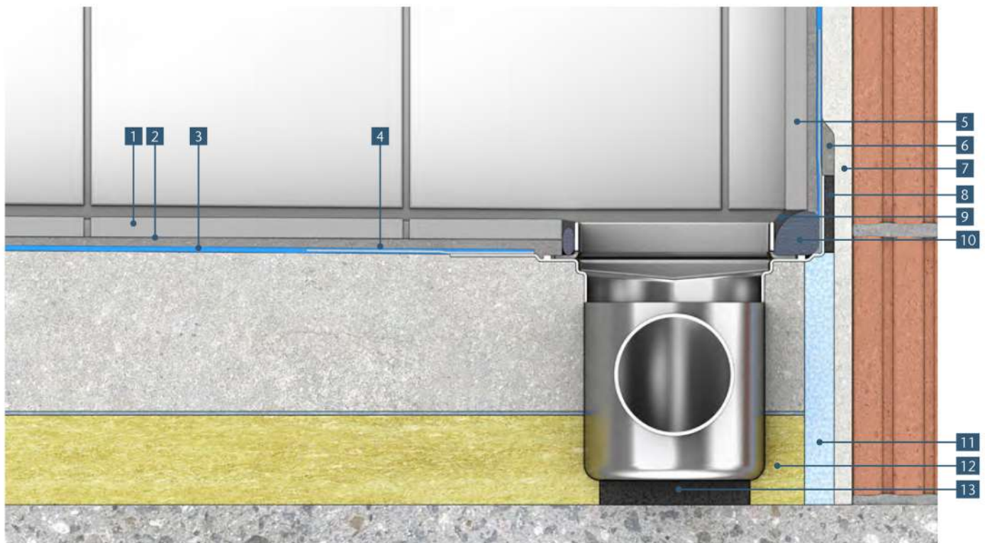
Installation proposal ACO ShowerDrain E+ (floor construction according sound insulation test report)
